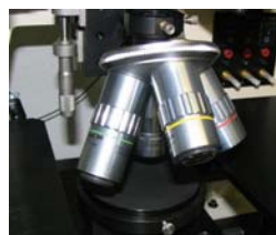
Optional 4-Position Objective Lens Turret
